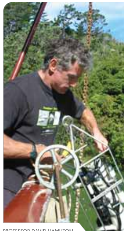
PROFESSOR DAVID HAMILTON MONITORS TEMPERATURE, OXYGEN AND ALGAL LEVELS IN THE WATER WITH A CTD PROFILER
